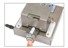
> Place the test strips into the strip holder.
