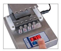
Move the strip holder into 2<sup>nd</sup> position and press the PUSH button on its back.
