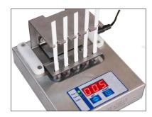
When Timer 1 finishes, the device beeps, on the display appears the time of Timer 2. The device automatically goes into Timer 2.
