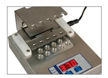
> Place the vials into the thermostatic device.
